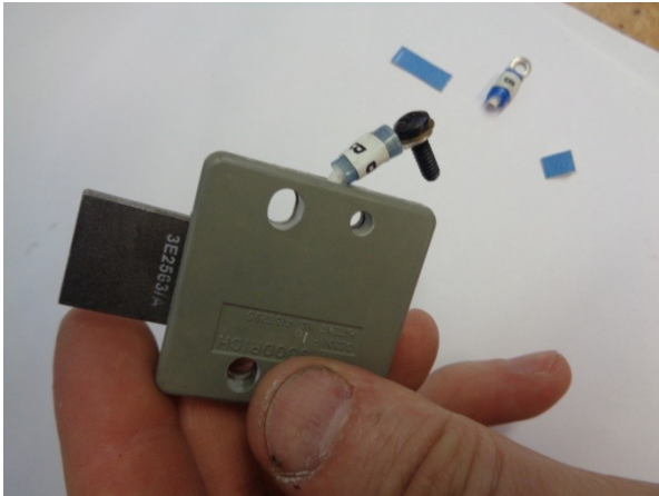
Fig.36 Remove the rubber band and release the brush; insert back all fasteners
