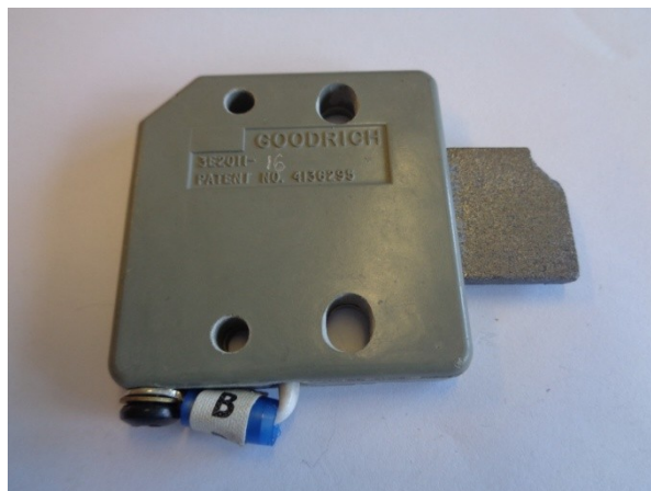
Fig.21 Brush module with damaged Brush
