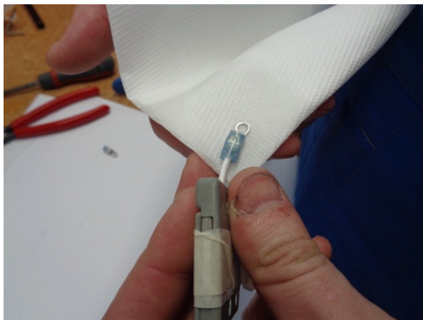
Fig.34 Ring terminal degreasing
