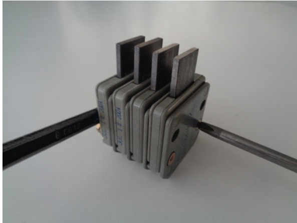
Fig.18 Remount Brush assembly on a flat and solid table
