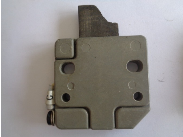
Fig.19 Brush module with damaged Brush
