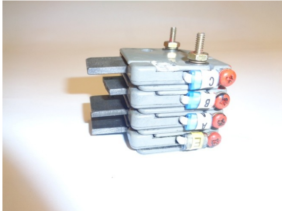
Fig.12 Damaged 4-races Brush assembly
