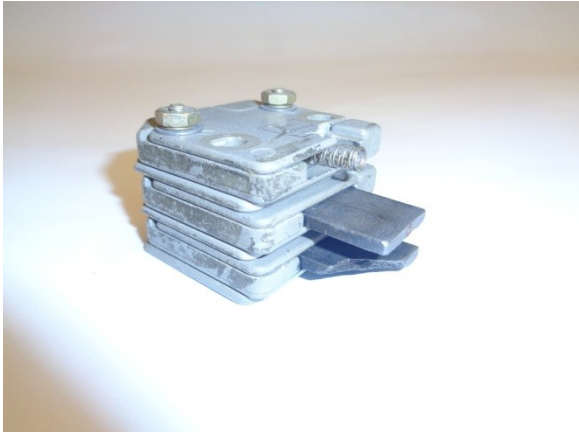
Fig.11 Damaged 3-races Brush assembly
